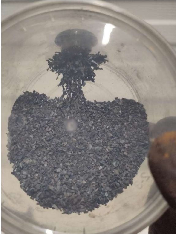
Direct Reduced Iron (DRI), which is magnetic, made by syngas from biomass.
