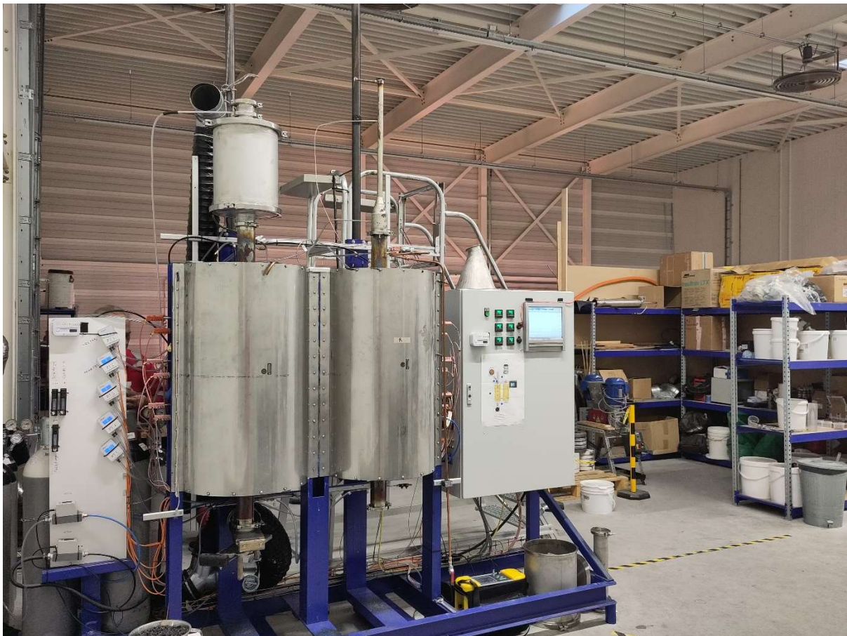
DOPS-RT test facility where syngas was made from biomass electrically.
