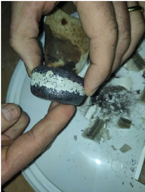
Iron made from low-grade ore, biomass, and electricity.
